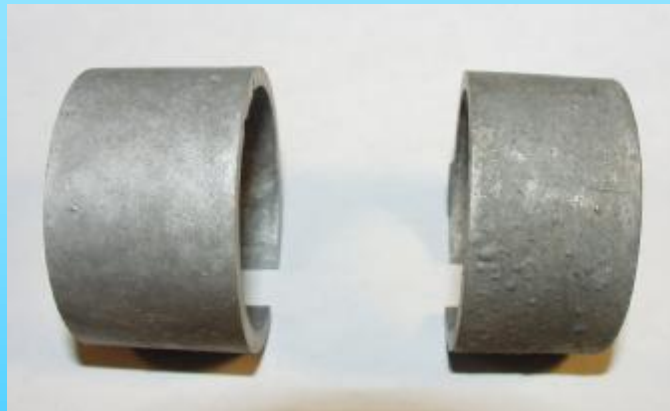
Blister Test of Semi-Solid and Liquid Die Cast Fuel Pump (520 °C)
